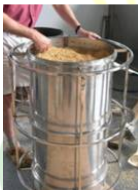
Figure. 2. The TLUD gasifier stove developed in Vietnam (Olivier, 2010)
